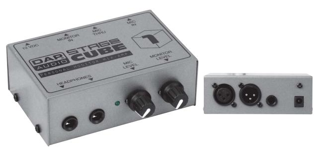
The SC-1 is a unique device for monitoring oneself and program material at the same time. It has a monitor level control and a mic level control, mic pass-through XLR jacks, two headphone output jacks, and a 1/4" monitor input jack. Possible users may be drummers who need to hear a click track, singers who need to hear themselves, etc. The power adapter is included.
